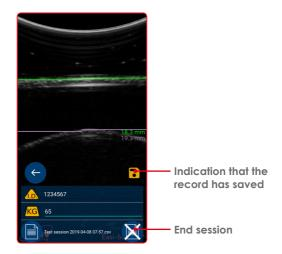
Each entry in the file will contain the animal id, weight, fat thickness, meat thickness, date and time, and the image reference for this measurement. The data is saved in a directory called BCFMQ.
