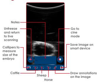
**Note:** Touch in the text area to type, up to 4 lines of text may be entered and will appear as red text with may be dragged to a preferred location. This text will be present on any saved images.
